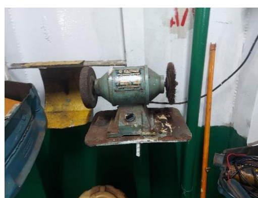
Safety Guards missing in Grinding Machine
