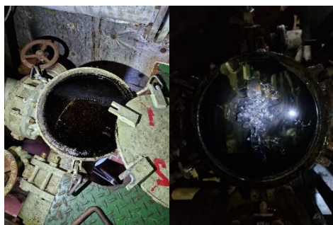
Bilge and ballast eductor suction filter and Fire & Bilge pump suction filter found with oil.
